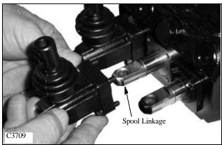
5 Pull out the spool. (fig. C3713) As you pull out the spool, note it's smooth action as it comes out of the valve body. The spool should move freely and smoothly in the bore of the valve body. Check the control valve spool and bore for scuff marks or abnormal wear. Replace the spool and or control valve if signs of wear are present.
