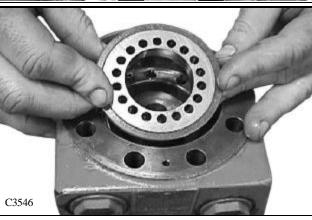
16 Example of an incorrectly installed balance plate. The guide pin becomes damaged and the balance plate is not locked into position. This can cause it to spin and render the motor non-functional (fig. C3547).
