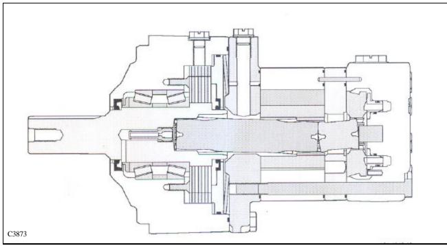
Fluid enters the housing through the inlet port and is directed to the balance plate. The balance ring contains an inner and outer seal to separate the high and low pressure fluid passages. Fluid passes through the stationary balance plate to the rotating disc valve. The rotating disc valve ports the fluid to the stationary valve plate and the proper side of the geroter pockets causing the rotor star to turn.
