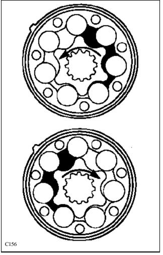
To seal the fluid pockets the torque motor incorporates a rotating roller type seal. (fig. C157) This type of a rolling seal reduces friction at the star points providing increased efficiency and reduced component wear.
