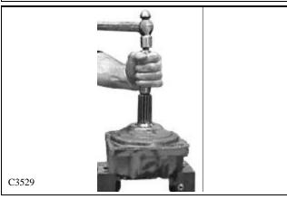
17 At this point the shaft should drop straight downwards. The shaft seal can now be removed and replaced. It can not be removed in any other way. (fig. C3530)
