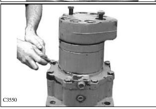
20 With ports all aligned, install balance of screws and tighten in a cross pattern, then final torque all bolts to 81 ft/lbs (fig. C3551).
