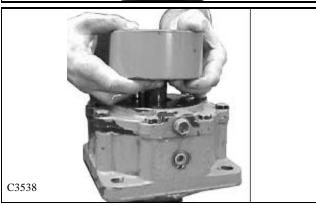
8 With the gearwheel mounted and the cardon shaft in place, place the drive gear valley to valley with the gearwheel. Mount the channel plate (ensuring the drain holes are aligned) and then valve drive it 15° counter clockwise (one tooth). Then mount the valve housing and re-install the bolts. (fig. C3539).
