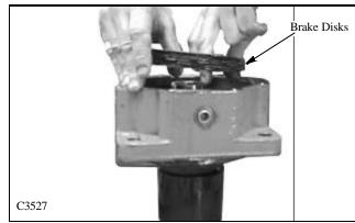
15 With the brake disks removed it exposes the shaft bearing retainer. Remove the eight (8) screws with a Torx driver. (fig. C3528)
