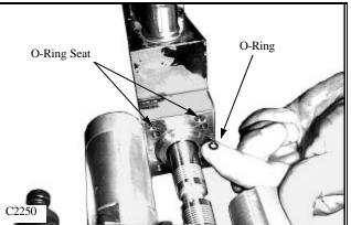
10 Upon assembly, use new O-ring seals. (fig. C3718) Don't over look the small O-ring seal between the cylinder and valve body. (fig. C2250) Lubricate the spool O-ring seals with system oil. Apply Castrol "Spheerol" grease to the inside of the spring covers.
