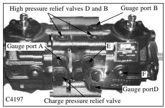
**NOTE:** Internal charge pump model shown
