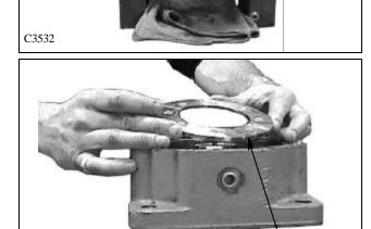
3 Alternate installation of brake disks, first putting in the outer disk (golden color) and then the inner disk (silver color). (fig. 3534)
