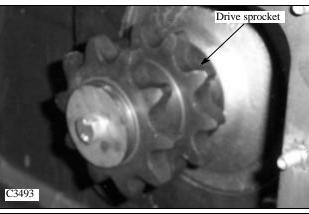
17 Install the sprocket, machined washer, lock washer and bolt. Apply Loctite 242 (blue) to the threads of the bolt before torquing (fig. C3767) and torque the bolt to  $40 \, \text{lbs} / \text{ft.}$  (54 nm).
