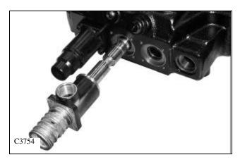
6 Remove the check valves from the control valve body (fig. C3757). They are located between the ports of each section. Check the seat and poppet of the valve body and check valve. Replace the check valve and/or the control valve if any signs of wear are present.
