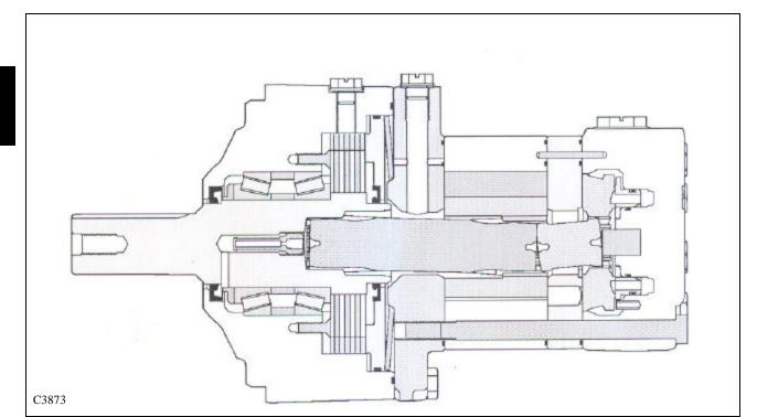
The basic geroter design uses a combination of mechanical and hydraulic principles that are utilized in the high torque, low speed motors.
