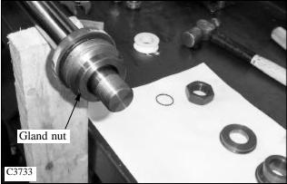
10 Remove and discard the wiper seal, rod seal and oring seals and teflon back up washer, (if used), from the gland nut assembly. (fig. C3734) NOTE: Some seal designs may vary from illustration
