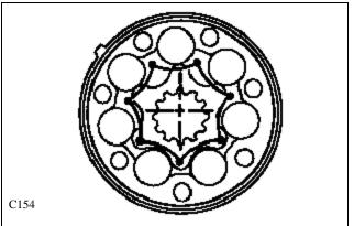
A drive shaft is used to transmit the rotation of the star to the output shaft. The drive shaft has crowned external splines to match the internal splines in the star and output shaft. This type of drive is used because the star center line continuously changes during rotation.
