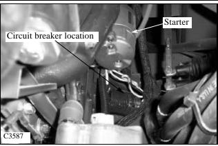
The loader is equipped with a 12 volt, negative ground electrical system. The fuse and relay panels are located in the engine compartment, attached to the underneath of the engine cover. (fig. C3588)
