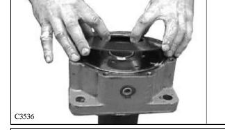
6 Install brake cover and cross tighten all screws to final torque specification of 65ft/lbs. (fig. C3537)
